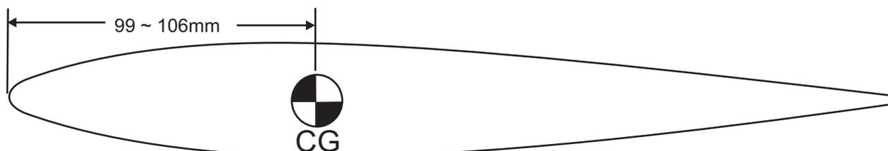
**WARNING !** Securely install the receiver and power pack, ensuring they will not come loose or rattle during flight. Never fly before checking the Cg's required position.
