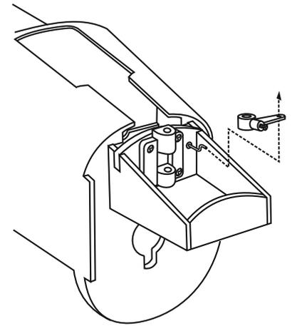
Insert the nose gear pushrod into the fuselage with the "Z" bend in front.
