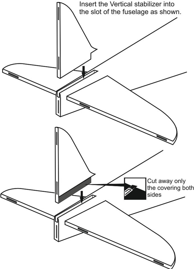
Glue the left and right of the vertical stabilizer, where it meets the fuselage
