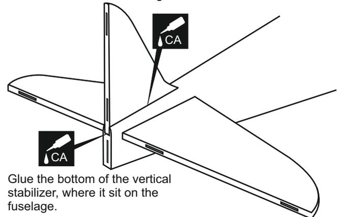
Glue the bottom of the vertical stabilizer, where it sit on the fuselage.
