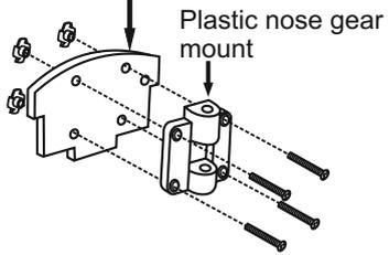
Attach the plastic nose gear mount to the plywood nose gear plate using four 3x20mm screws and blind nuts.
