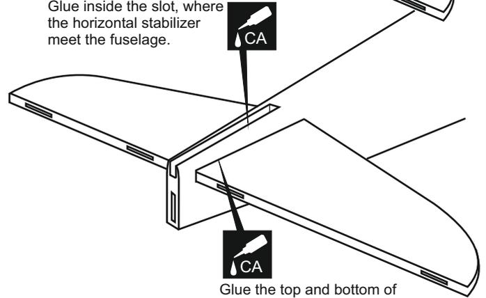
Glue the top and bottom of the horizontal stabilizer, where it meets the fuselage
