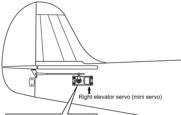
Apply a thin layer of machine oil or petroleum jelly to only the **top and bottom of the trailing edge of the elevator**, then push the elevator and its hinges into the hinge slots in the trailing edge of the horizontal stabilizer. When satisfied with the alignment, hinge the elevator to the horizontal stabilizer using CA glue. Do the same way with the rudder.
