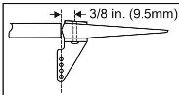
When you are satisfied with the alignment of the control horn mark the mounting hole positions with a felt tipped pen or a pencil. Remove the control horn and drill two 2mm (5/64") holes through the rudder and elevator. Attach the rudder and elevators control horn using two 5/64X15/32"(2x12mm) screws and a back plate.
