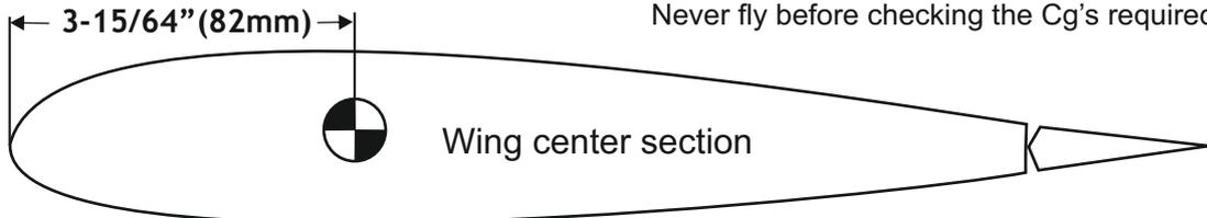
In order to obtain the CG specified, reposition the receiver and power pack
