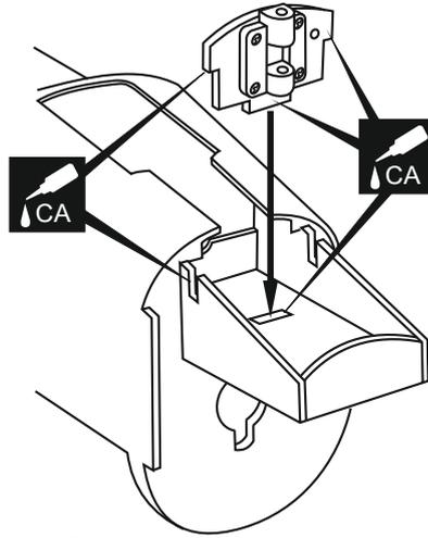
Secure the plywood nose gear plate in place using CA glue.
