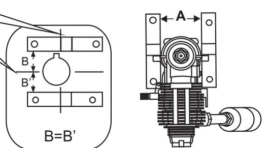
Using a pencil or felt tipped pen, mark the fire wall where the four holes are to be drilled.
