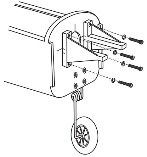
Position the engine on to the engine mounts so the distance from the prop hub to the fire-wall is 5.2"(132mm). Mark the engine mounting plate where the four holes are to be drilled.
