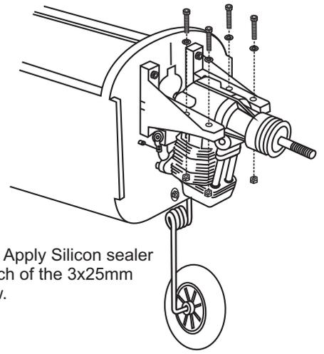
Note: Mark the mounting plate through the engine mounting flanges.
