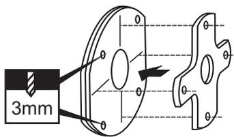
Using an aluminum motor mounting plate as a template, mark the plywood motor mounting plate where the four holes are to be drilled.
