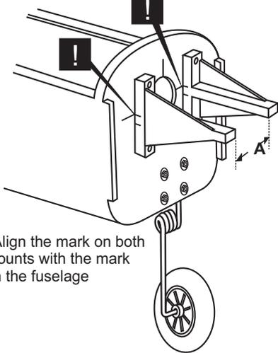
! Align the mark on both mounts with the mark on the fuselage
