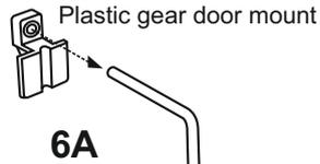
**6A** Slide the two plastic gear door mounts onto each landing gear.
