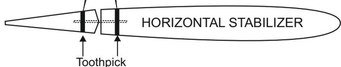
Cut the excess toothpick and secure it in place using little Thin CA glue.
