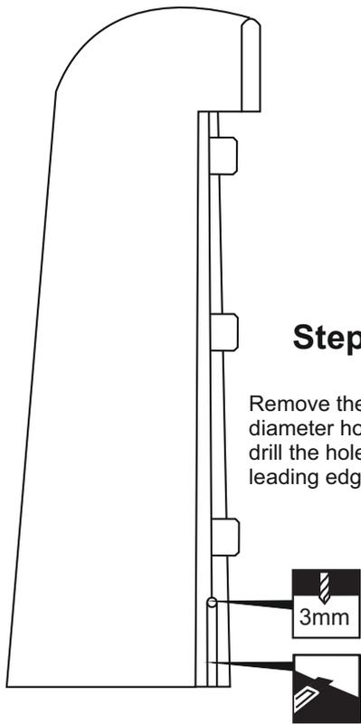
Cut the rudder torque rod mounting slot.
