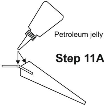
Apply a thin layer of machine oil or petroleum jelly to only the pivot point and the leading edge of the elevator.
