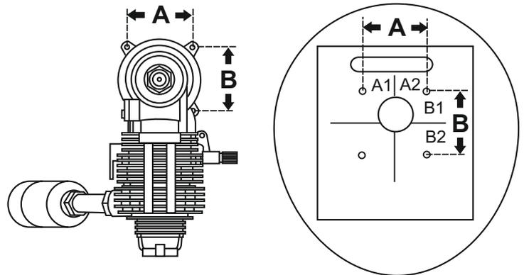
Mark the plywood where the four holes are to be drilled.
