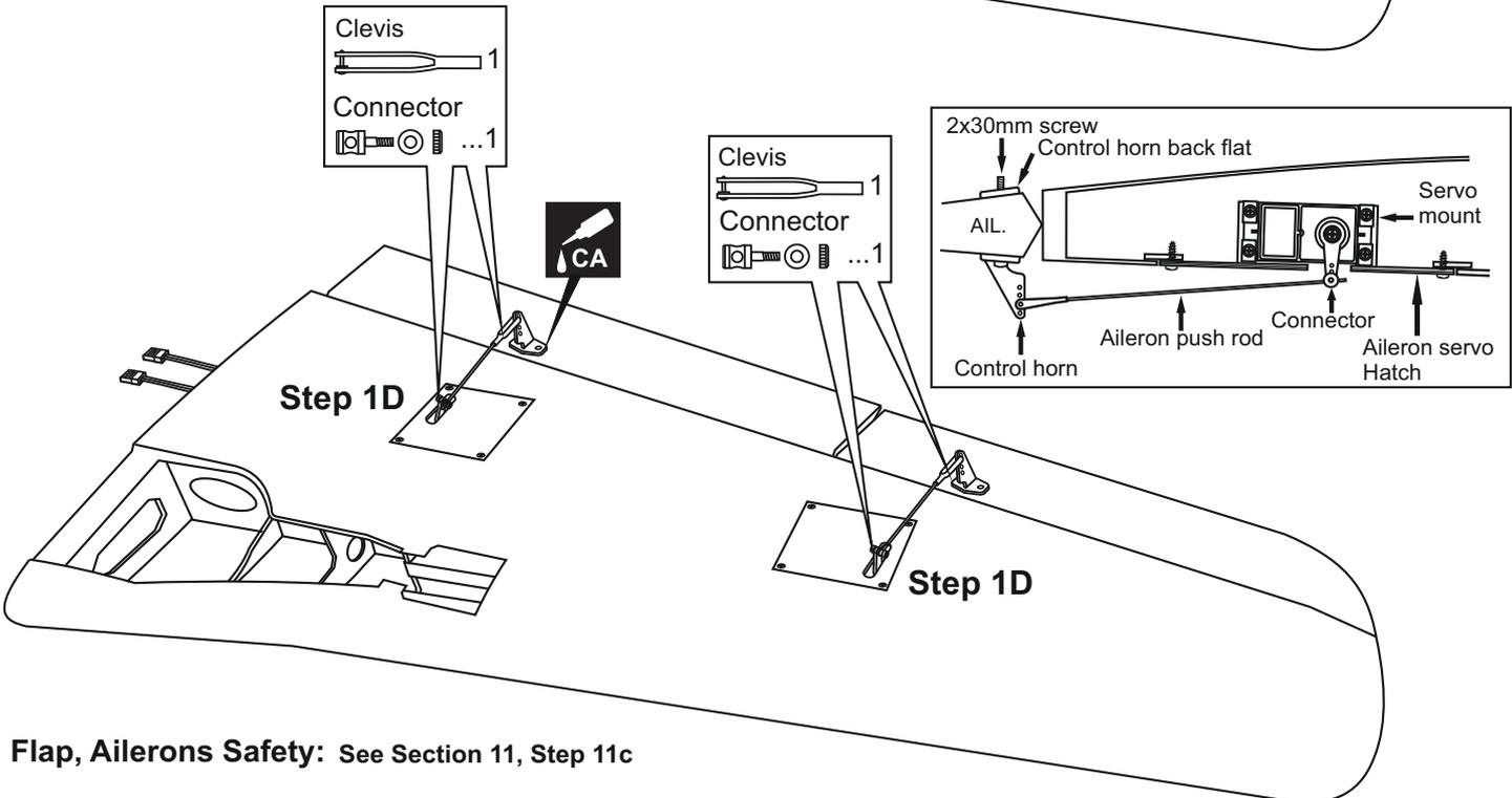
Flap, Ailerons Safety: See Section 11, Step 11c
