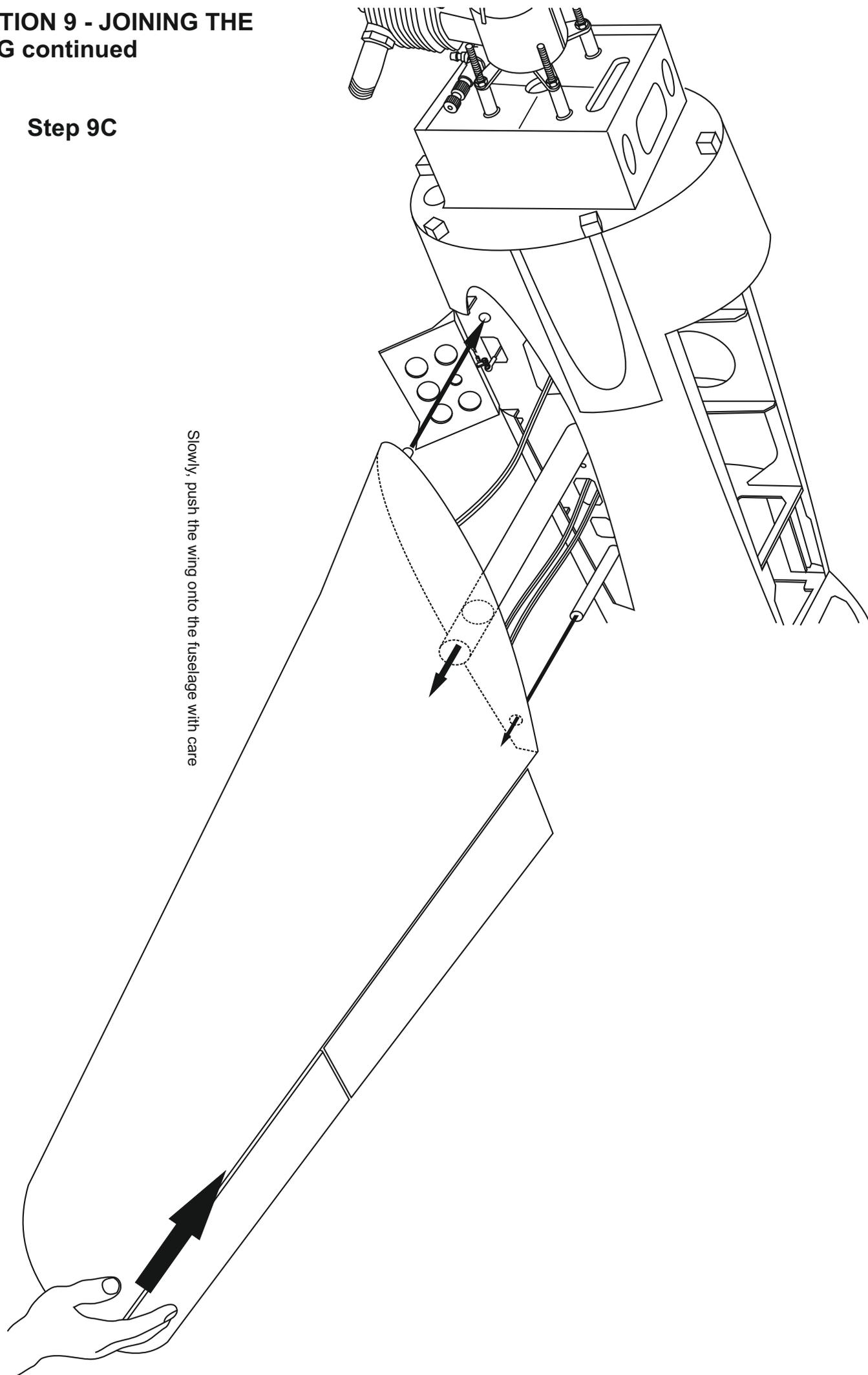
Slowly, push the wing onto the fuselage with care
