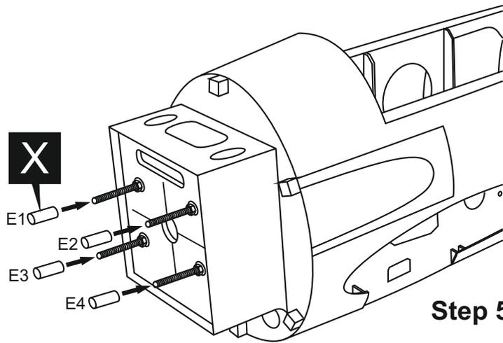
E1=E2=E3=E4 (The long of the aluminum tubes are the same and depend of your engine)
