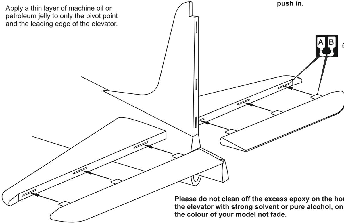
Please do not clean off the excess epoxy on the horizontal stabilizer and the elevator with strong solvent or pure alcohol, only use kerosene to keep the colour of your model not fade.
