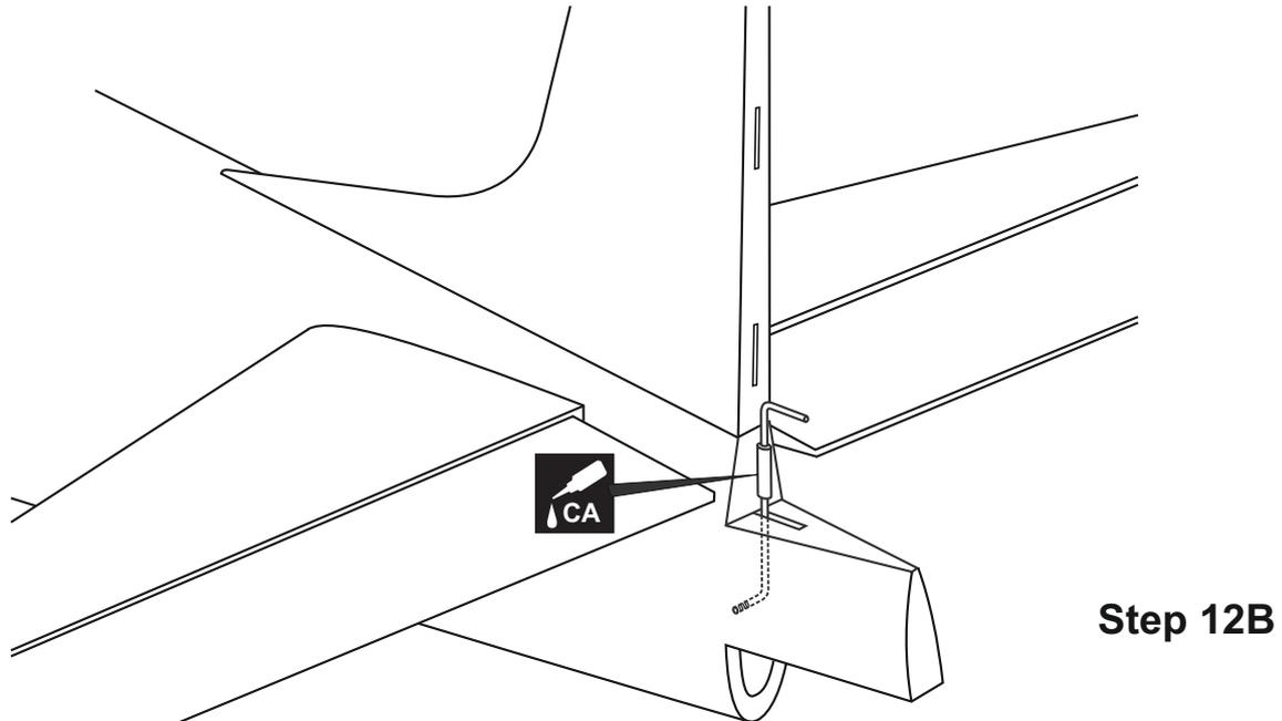
Glue the rudder torque rod bearing into the slot you cut previously in the vertical stabilizer Using the thin CA glue.
