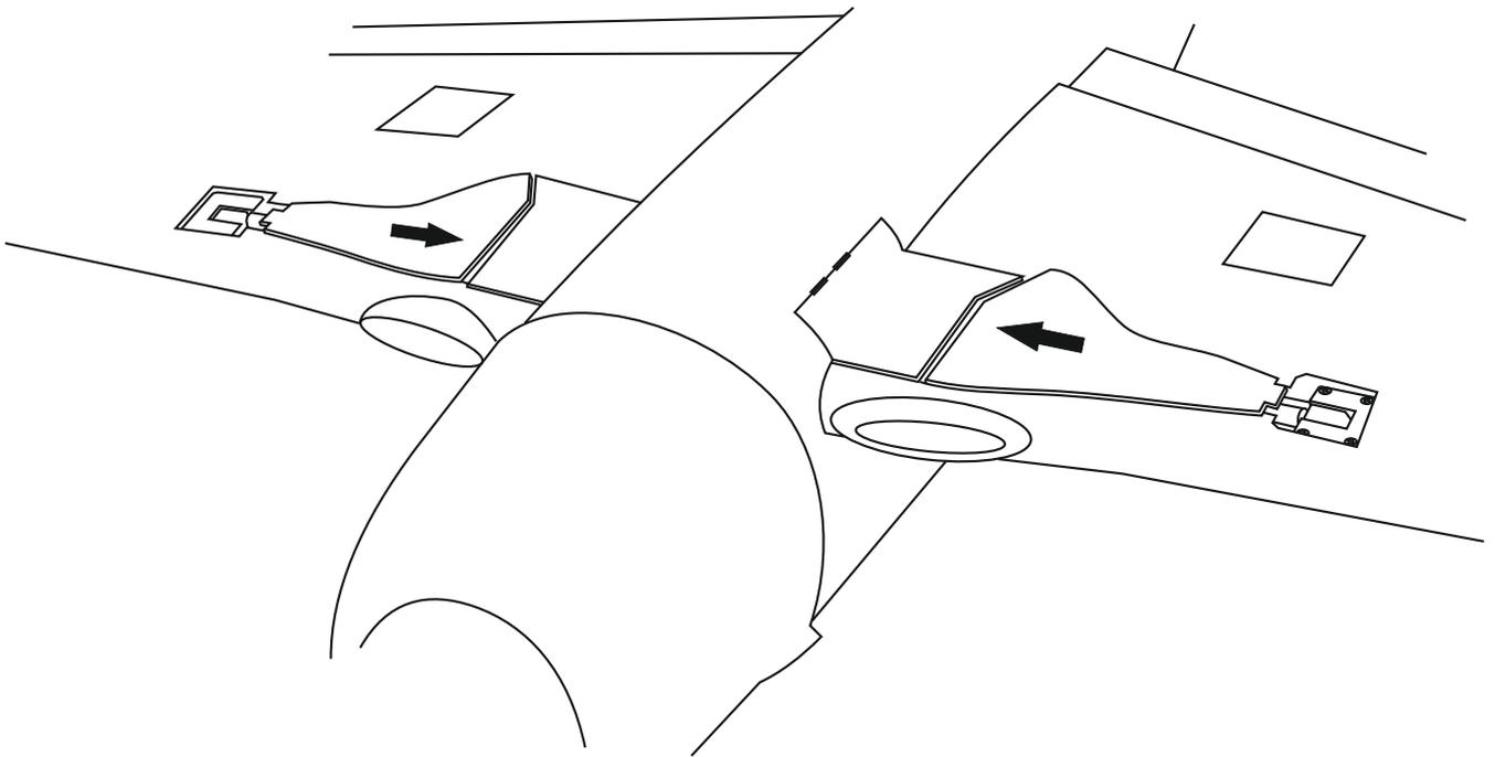
With the retract in the retracted position, carefully move the gear door on the strut until the gear door nearest with the gear door on the fuselage, mark on the struts.
