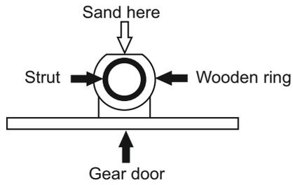
Lightly sand the wooden rings to be sure that the struts locks in down position.
