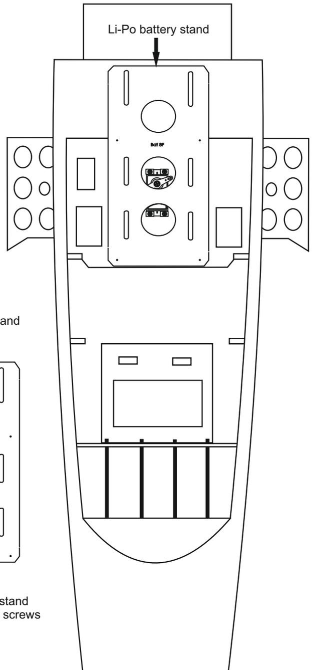
Secure the battery stand using four 3x10mm screws
