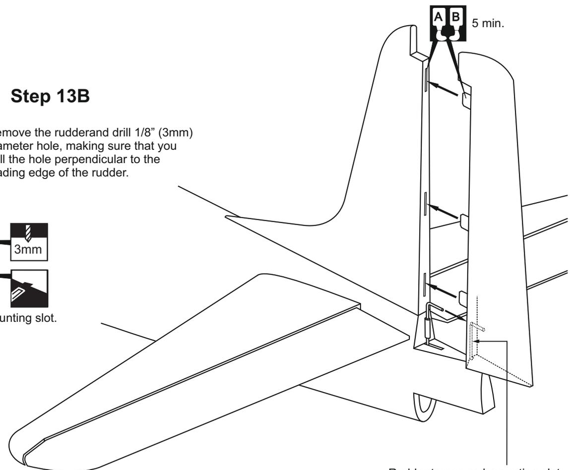
Rudder torque rod mounting slot
