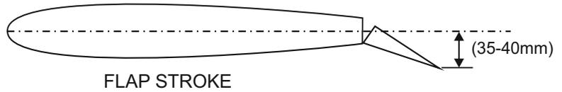
Adjust the travel of the control surfaces to achieve the values stated in the diagrams.
