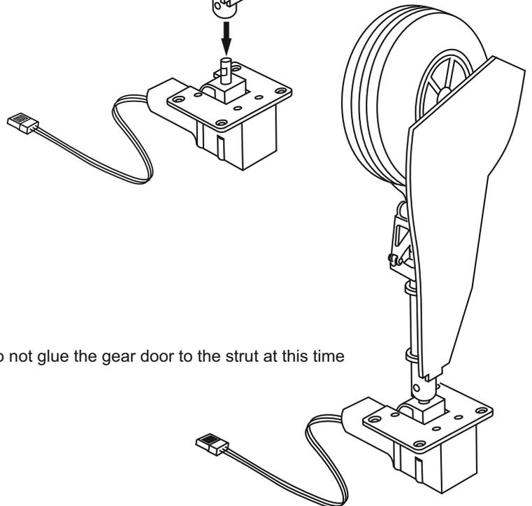
Note: Do not glue the gear door to the strut at this time
