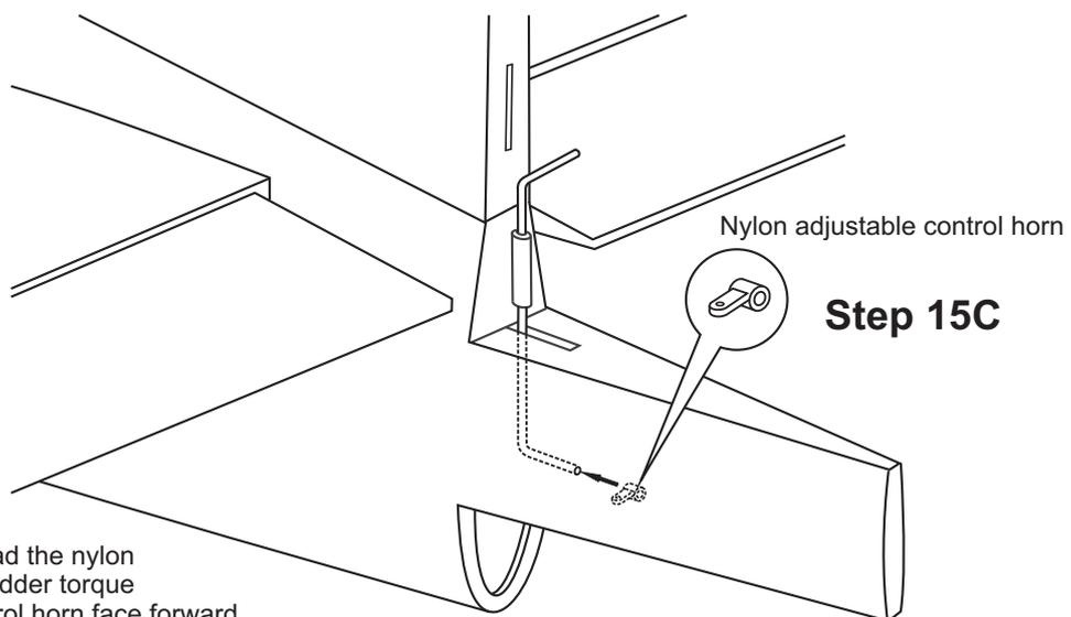
Turn the rudder torque rod bearing, Thread the nylon adjustable control horn onto the end of rudder torque rod, making sure that the adjustable control horn face forward.
