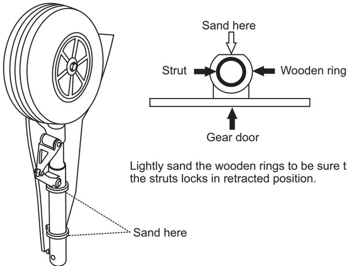
Lightly sand the wooden rings to be sure that the struts locks in retracted position.
