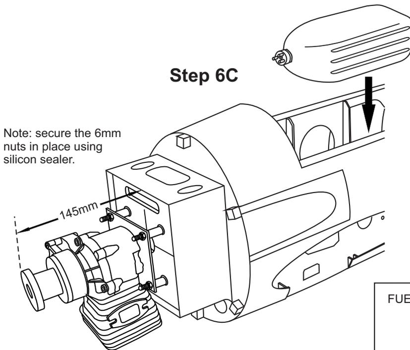
Note: secure the 6mm nuts in place using silicon sealer.
