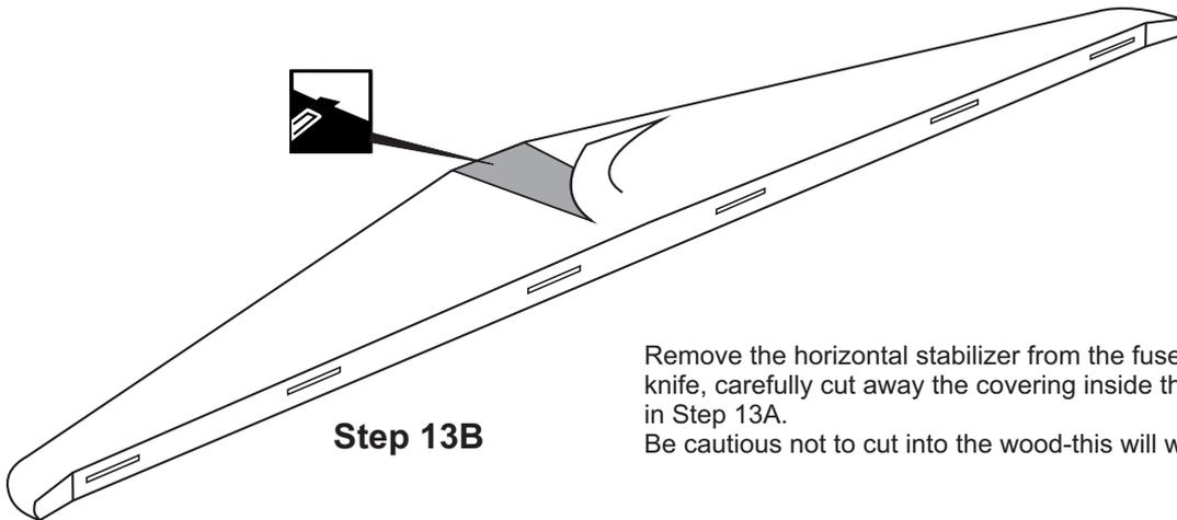
Remove the horizontal stabilizer from the fuselage. Using a sharp hobby knife, carefully cut away the covering inside the lines which were marked in Step 13A. Be cautious not to cut into the wood-this will weaken the structure.
