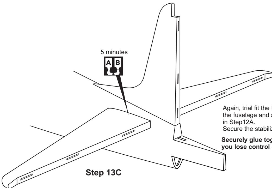
Again, trial fit the horizontal stabilizer in place on the fuselage and adjust the alignment as described in Step 12A. Secure the stabilizer in place using the 5 minutes Epoxy.
