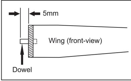
Glue the dowel to the rib root, marking sure that the dowel perpendicular to surface of the rib root.
