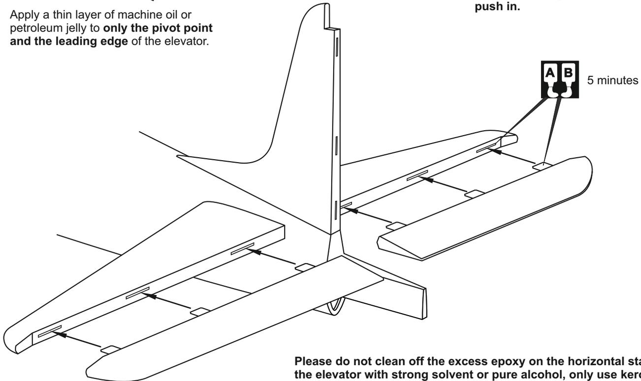
Please do not clean off the excess epoxy on the horizontal stabilizer and the elevator with strong solvent or pure alcohol, only use kerosene to keep the colour of your model not fade.
