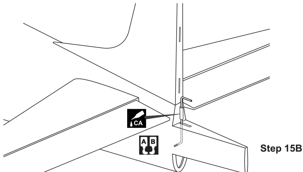
Glue the rudder torque rod bearing into the slot you cut previously in the vertical stabilizer Using the thin CA glue.
