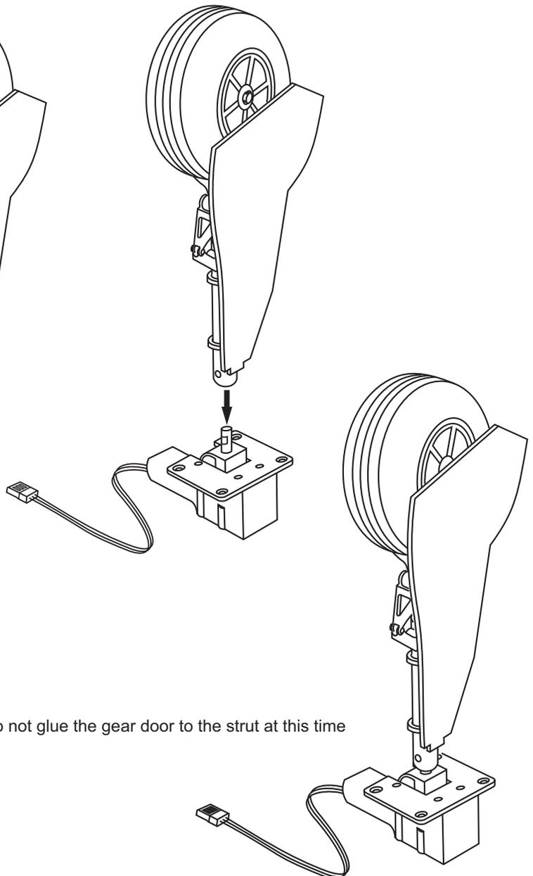
Note: Do not glue the gear door to the strut at this time
