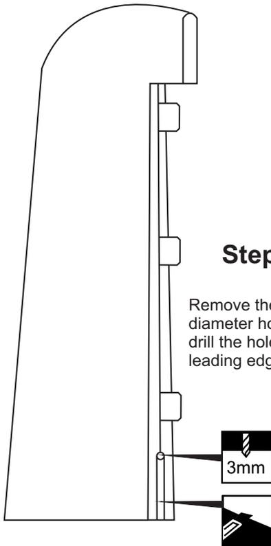
Cut the rudder torque rod mounting slot.
