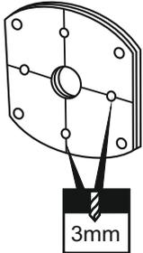
Remove the aluminum motor mounting plate and drill a 1/8" (3mm) hole through the plywood at each of the four marks marked.
