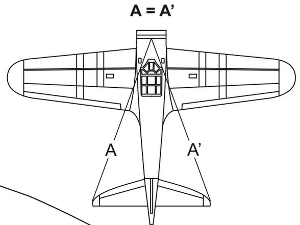
When you are satisfied with the alignment, use a pencil to trace around the top and bottom of the stabilizer where it meets the fuselage (13B).
