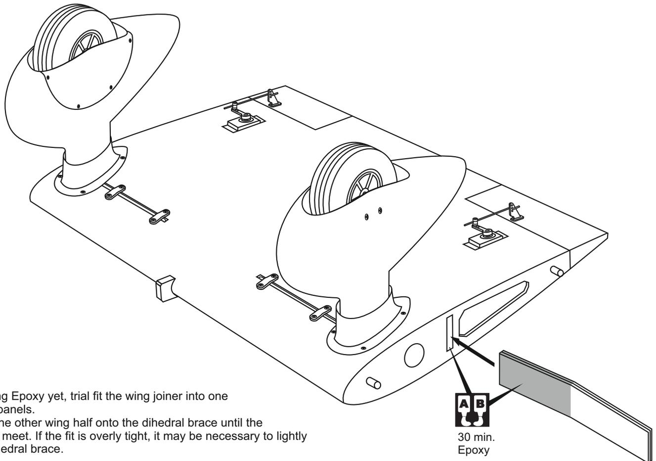
Without using Epoxy yet, trial fit the wing joiner into one of the wing panels.
