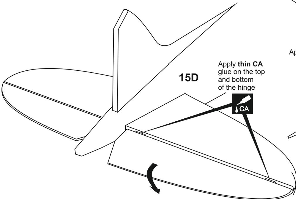
Apply thin CA glue on the top and bottom of the hinge
