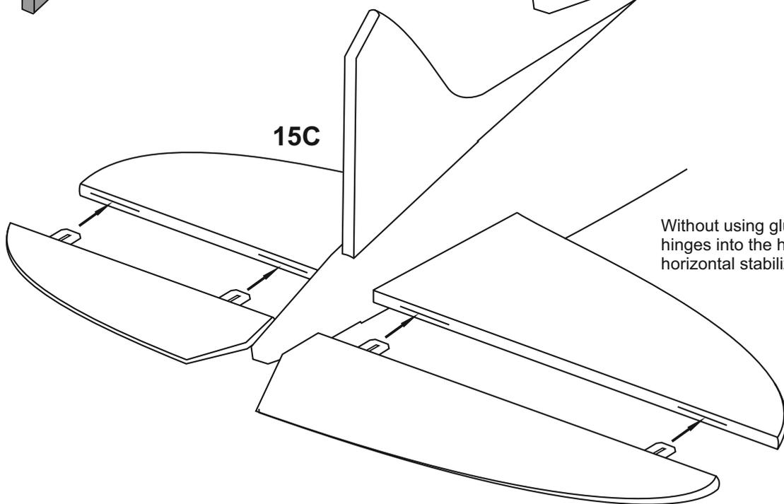
Without using glue yet, push the elevator and its hinges into the hinge slots in trailing edge of the horizontal stabilizer (15C).
