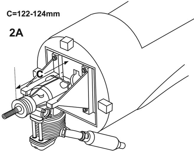
Position the engine to the engine mounts so the distance from the prop hub to the fire-wall is 122 - 124mm.
