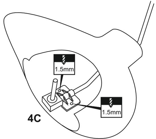
Remove the clothespin and drill the two 1.5mm holes as shown (4C).
