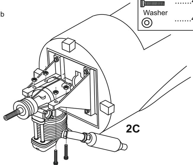
Reposition the engine on the engine mount beams, aligning it with the holes. Secure the engine to the engine mount using four 3x25mm screws (2C)
