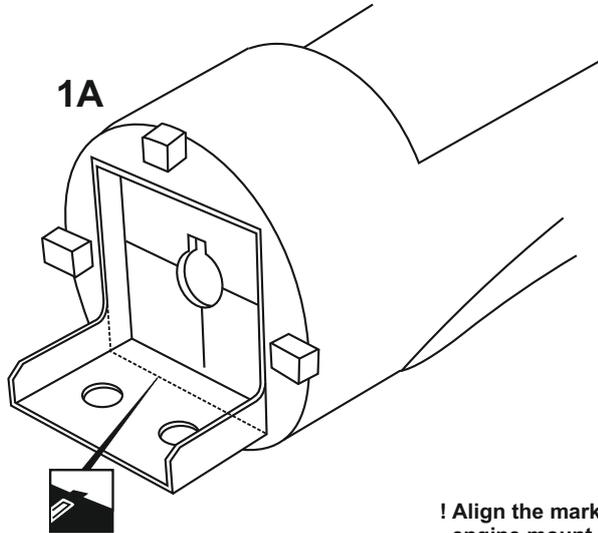
Attach the engine mount beams onto the fire-wall so the distance between of two engine mount beams is "A", and B=B' as show.
