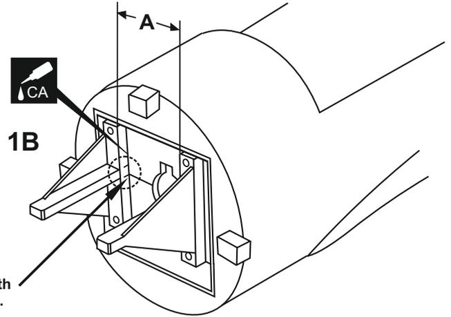
**! Align the mark on both engine mount beams with the mark on the fire-wall.**
