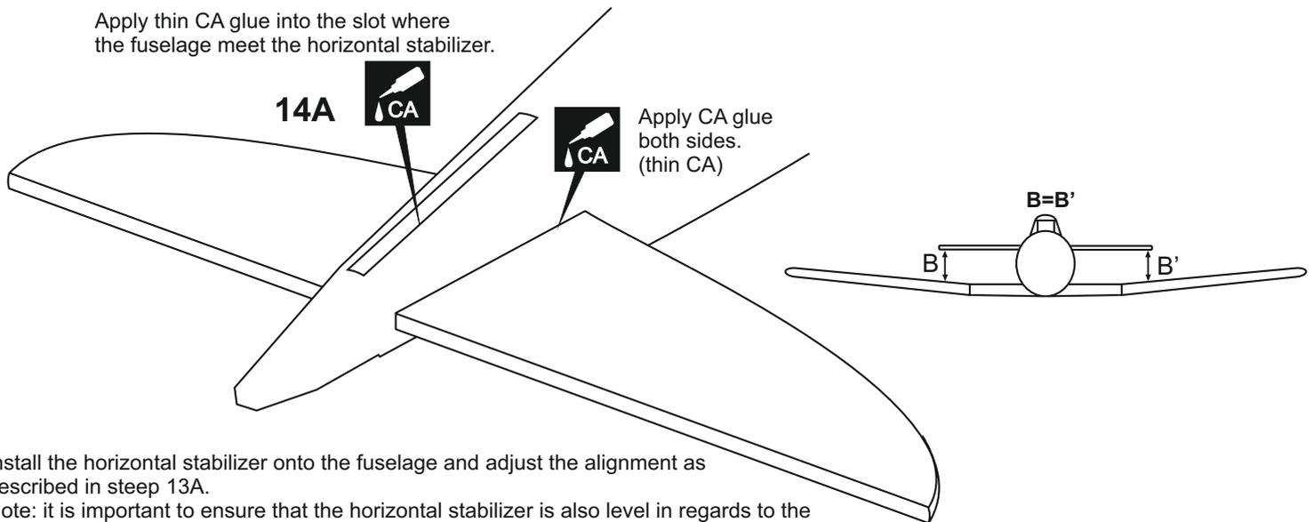
Install the horizontal stabilizer onto the fuselage and adjust the alignment as described in steep 13A.
