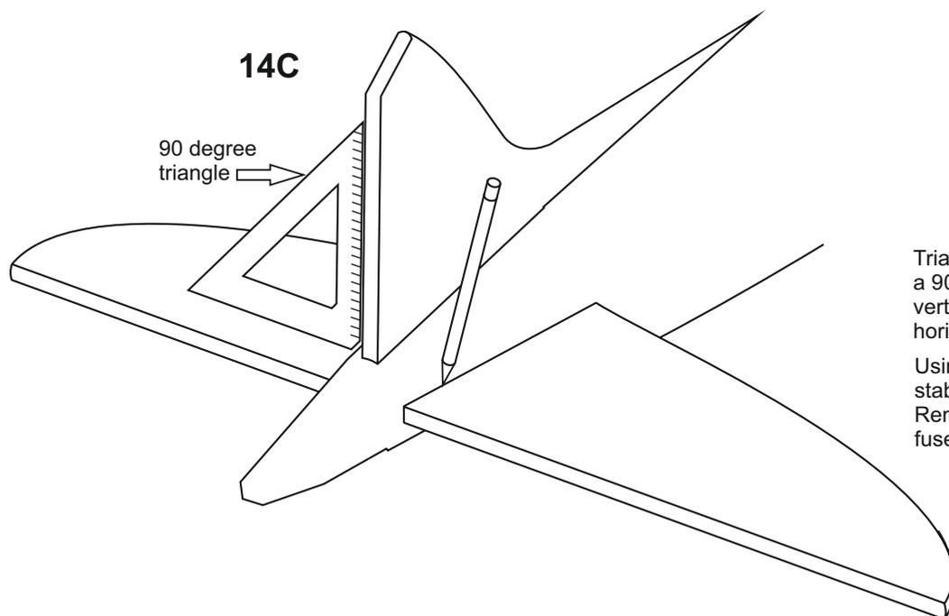
Trial fit the vertical fin in position. Using a 90 degree triangle, ensure that the vertical stabilizer is perpendicular to the horizontal stabilizer (14C).
