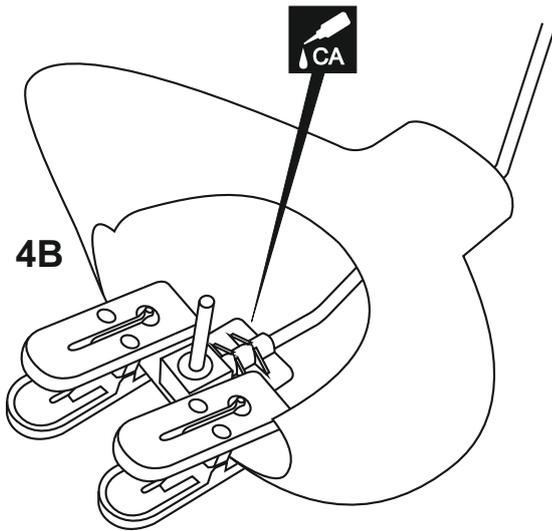
Slide the landing gear with the wheel pant into the fiber glass wheel pant and secure it in place using the two clothespin and litter thin CA glue as shown (4B).
