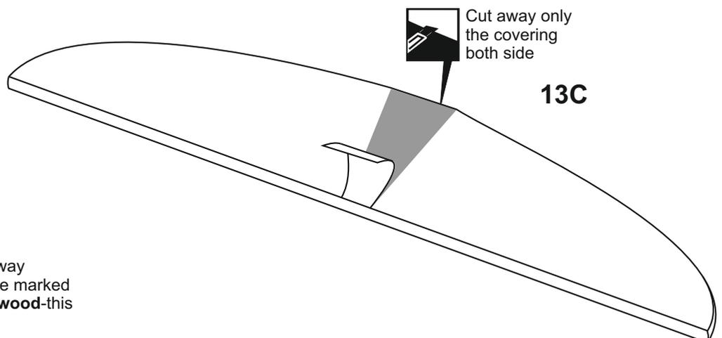
Remove the horizontal stabilizer from the fuselage. Using a straight edge and a sharp hobby knife, carefully cut away the covering **inside the lines** which were marked above. Be cautious **not to cut into the wood**-this will weaken the structure (13C).
