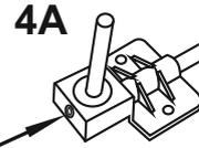
Secure the wheel pant mount in place using the 3mm screw set.
