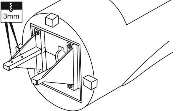
Remove the engine and drill a 3mm holes through the beam at each of the four marks made above (2B)
