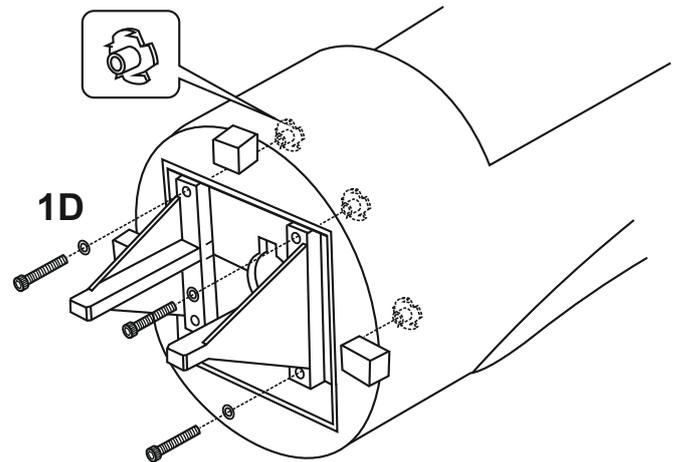
Insert the blind-nut onto each of the four holes make above (1D).
