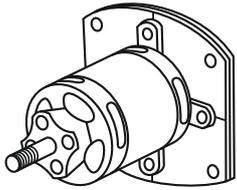
Using an aluminum motor mounting plate as a template, mark the plywood motor mounting plate where the four holes are to be drilled.
