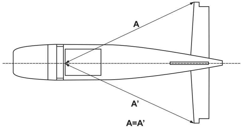
When you are satisfied with the alignment, use a pencil to trace around the top and bottom of the stabilizer where it meets the fuselage.
