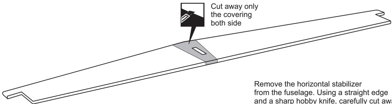
Remove the horizontal stabilizer from the fuselage. Using a straight edge and a sharp hobby knife, carefully cut away the covering **inside the lines** which were marked above. Be cautious **not to cut into the wood**-this will weaken the structure.
