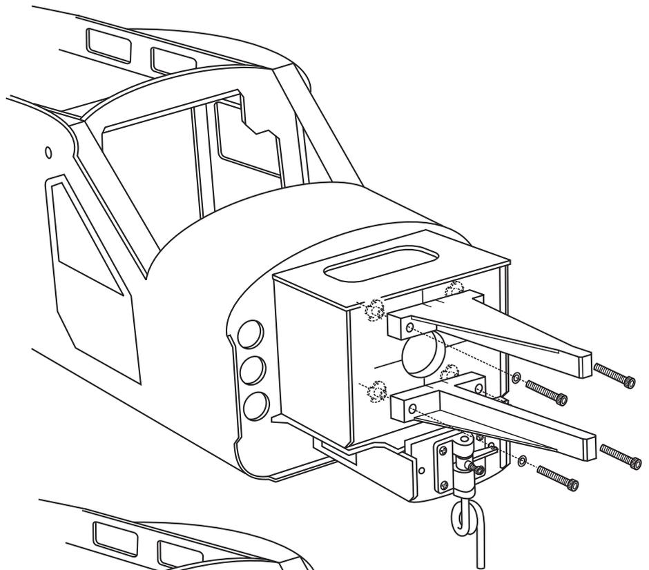
Position the engine to the engine mounts so the distance from the prop hub to the fire-wall is 130mm.
