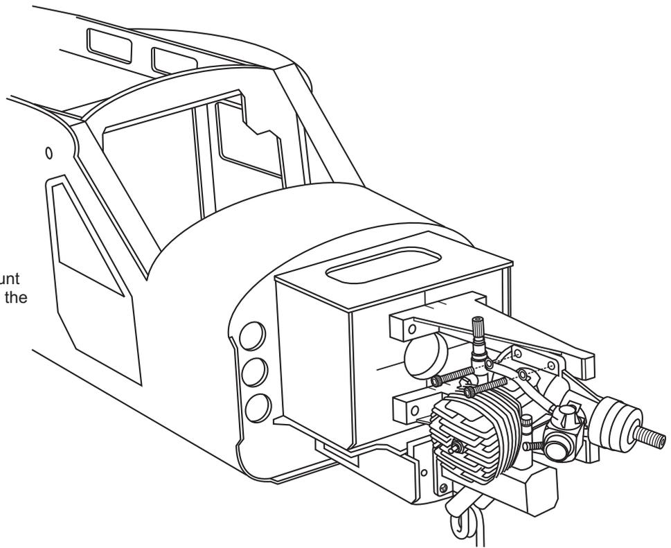
Reposition the engine on the engine mount beams, aligning it with the holes. Secure the engine to the engine mount using four 3x25mm screws.
