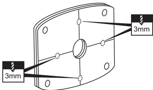
Remove the aluminum motor mounting plate and drill a 3mm hole through the plywood at each of the four marks marked .
