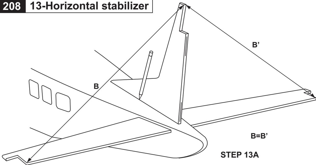
Trial fit the vertical fin in position. Using a 90 degree triangle or adjust the vertical stabilizer ensure that the B=B' as shown, the vertical stabilizer is perpendicular to the horizontal stabilizer.
