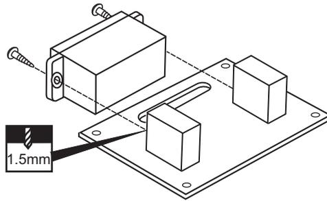
FLAP SERVO HATCH - TOP VIEW
