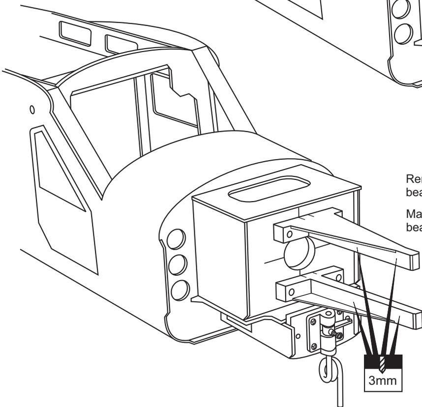
Remove the engine and drill a 3mm holes through the beam at each of the four marks made above.
