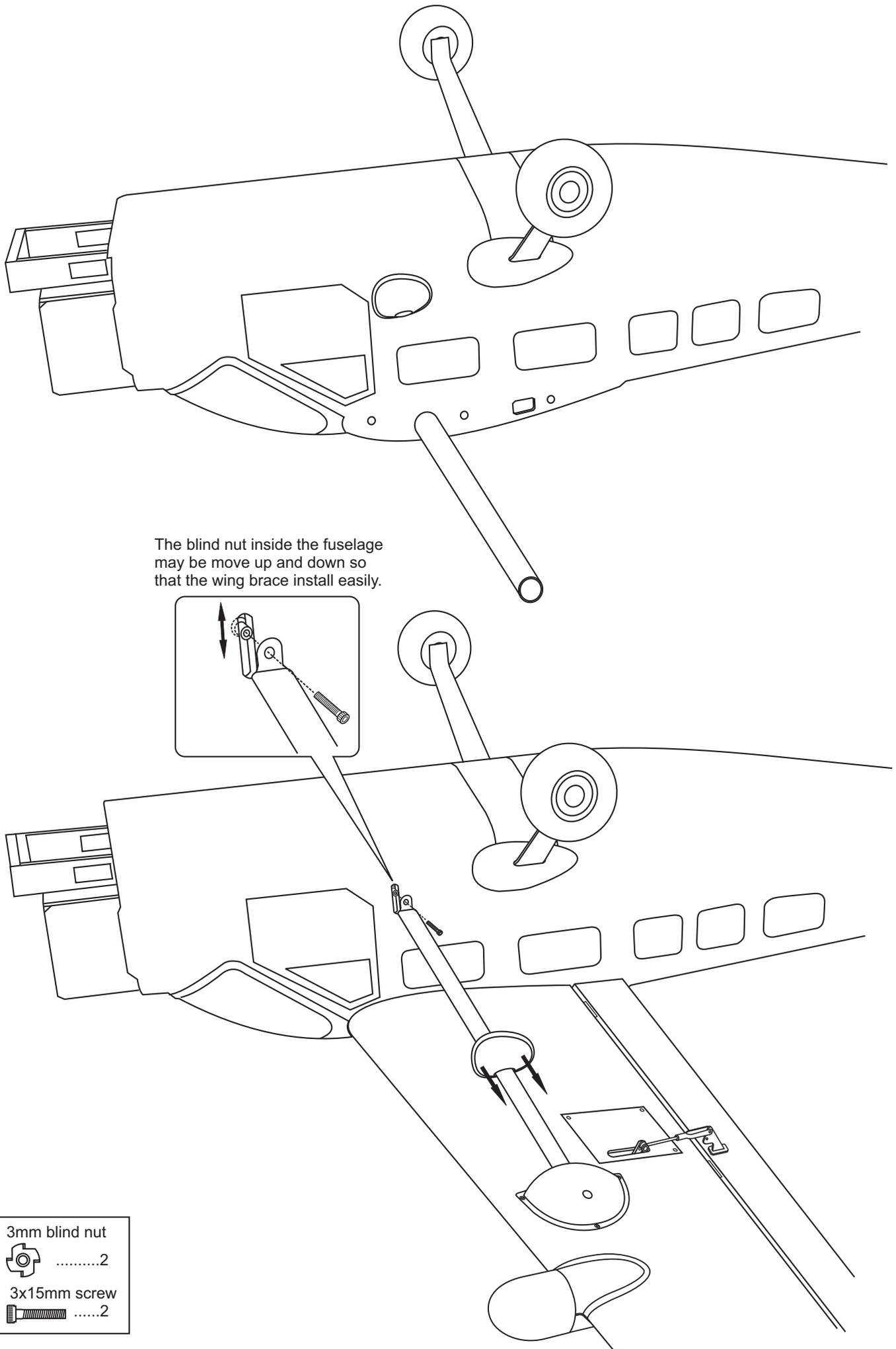
The blind nut inside the fuselage may be move up and down so that the wing brace install easily.
