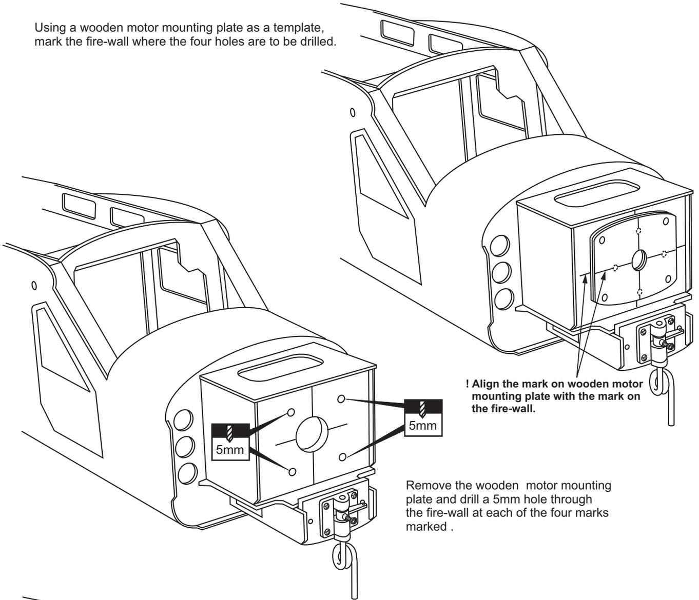
**! Align the mark on wooden motor mounting plate with the mark on the fire-wall.**
